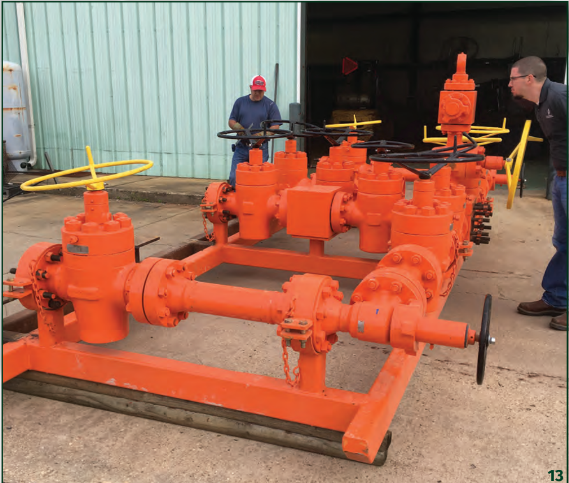
REFURBISHED DRILLING MANIFOLD
